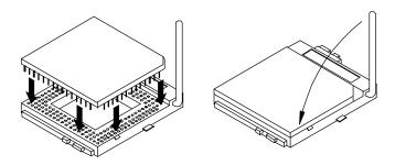
After you have installed the processor into the socket, check if the jumpers for the CPU type and speed are correct.
